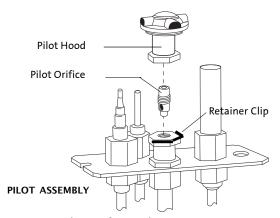
Figure 13. Pilot Orifice replacement.
